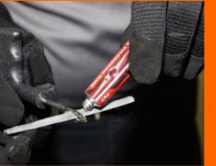
2. Apply a small amount of Chemical Vulcanizing Fluid to the Reaming Tool and then apply to the puncture using an in/out motion. Leave the Reaming Tool in the tire for now.
