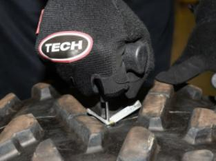
5. Remove the Installation Tool by pulling straight out of the tire.
