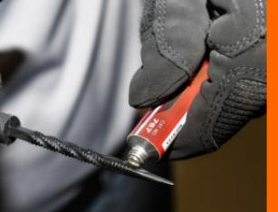
4. Remove the Reaming Tool from the tire. WITHOUT TWISTING the Installation Tool, push the PermaCure insert into the tire until the loop of the PermaCure clears the inside of the tire.
