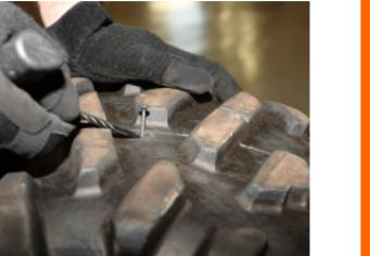
3. Remove the blue protective cover from the PermaCure. Do not touch the PermaCure. Insert the PermaCure into the eye of the Installation Tool and apply a light coat of Chemical Vulcanizing Fluid.
